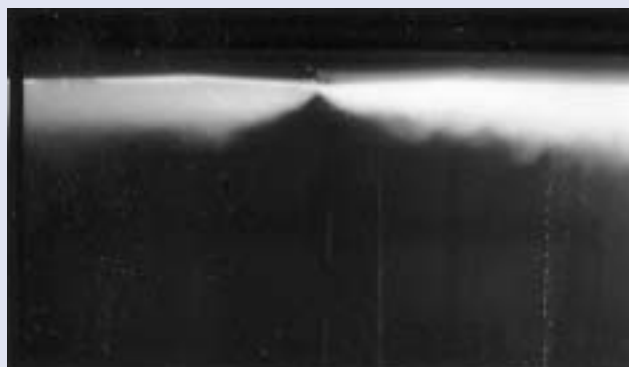
Photo 3: VSD-1-Varyset, \dot{V} = 22 \text{ l/s} ; \Delta t = - 8 \text{ K}
