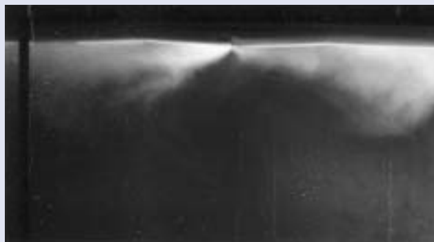
Photo 4: VSD-1-Varyset, \dot{V} = 11 \text{ l/s} ; \Delta t = - 8 \text{ K}
